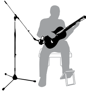
Figure 7: Miking an acoustic guitar with a single C214
